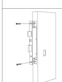
Insert the screw into the hole and fix it
