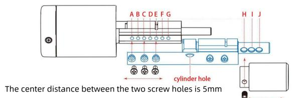
• Change the length of the cylinder by adjusting the position of the screw inserted into the screw hole.
