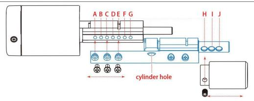
Adjust the length of the cylinder according to the door thickness
