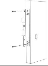
Insert the screw into the hole and fix it.
