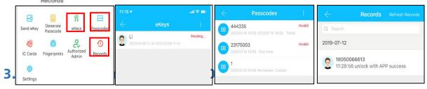
The TT lock is directly connected via Bluetooth, that is why it is not attacked by the network. The gateway is a bridge between smart locks and home WIFI networks. Through the gateway, the user can remotely view and calibrate the lock clock, read the unlock record. Meanwhile, it can remotely delete and modify the password.
