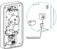
3 After the access control is powered on: Long press the reset button to hear "please input initialization pass-code" enter: 000#, with sound: "Successful". Then the lock is under factory state, the default master password is: 123456 with # to confirm. you can open the door with any fingerprint.
